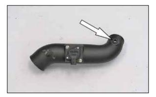
18. Install the mass air sensor assembly into the K&N® intake tube as shown and secure with the provided hardware. Install the crank case vent grommet into the K&N® intake tube as shown. NOTE: The arrow on the top of the sensor indicates the direction of air flow when the sensor is installed correctly.
